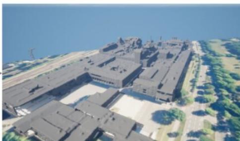
Fusion with LiDAR data scans increases resolution to 10 cm
