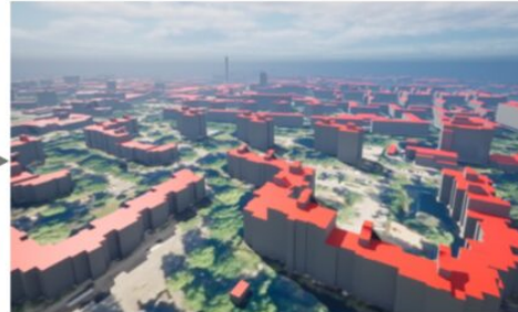
Structure of buildings is reconstructed based on public registry data, including type of building material and other features as available
