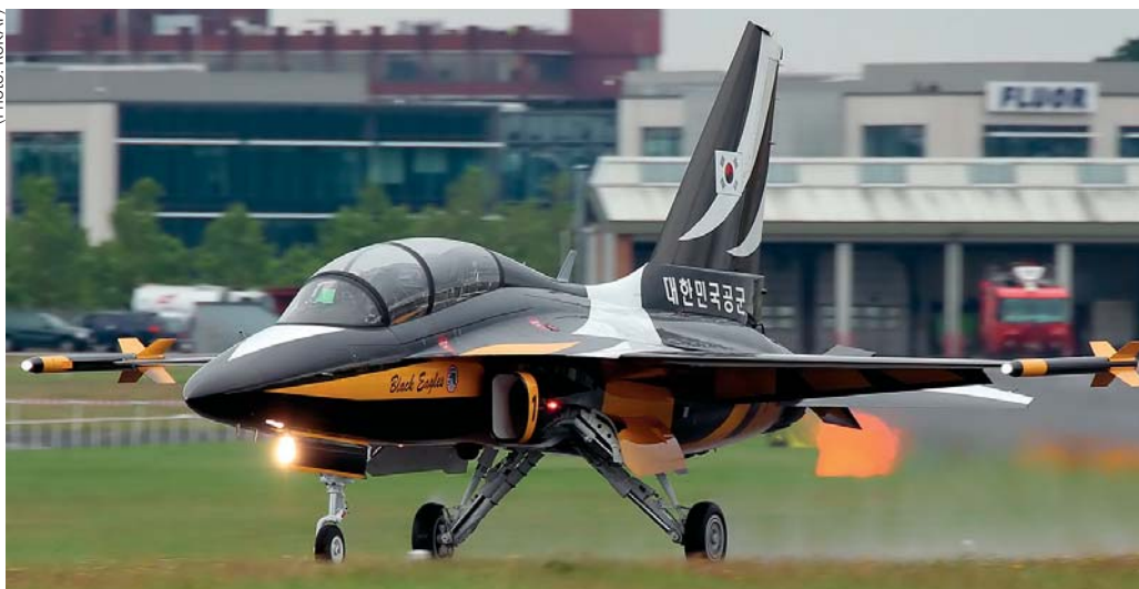
The T-50 Golden Eagle is a family of South Korean supersonic advanced trainers and multirole light fighters, developed by the consortium that was established by Korea Aerospace Industries (KAI) along with the American aerospace company Lockheed Martin.
